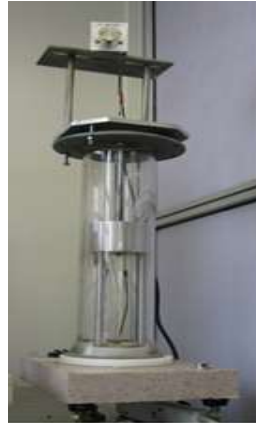
Figure 2-17: Photo illustrates Travelling heater method [2.36].
