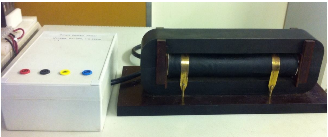
Figure 4.1 Single strip tester for measuring the power loss.
