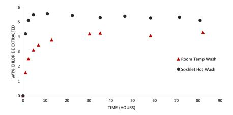
greater than for the Soxhlet hot-washed samples. Rinsing the Soxhlet hot-washed sample does not reduce its oxygen consumption rate below the unrinsed sample. This is reflected in the very small amount of extra Cl removed in the rinse process (Table 1). There is good agreement between the corrosion rates for the samples washed in the same manner, demonstrating reproducibility in the oxygen consumption measurement method.
