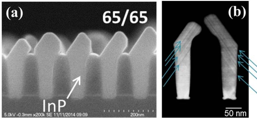
286 **Figure 3.** (a) SEM image of a cross section along  $[1\bar{1}0]$  of InP fins selectively grown in 180
