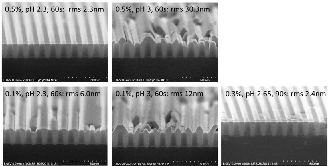
303 **Figure 7.** Tilt cross-section SEM images of test structure post InP CMP.
