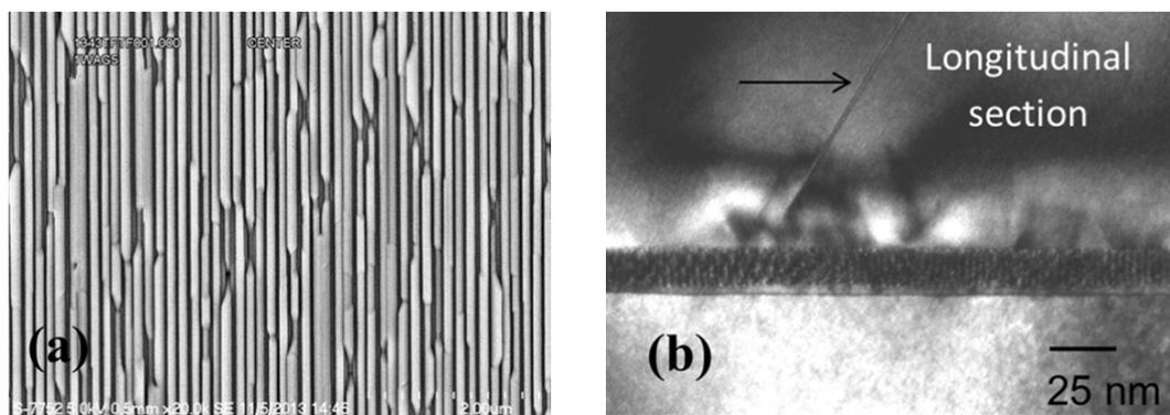
282 **Figure 2.** (a) Top-down view SEM image of InP fins on Si (001); (b) TEM image of a cross
