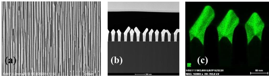
291 **Figure 4.** (a) Top-down view SEM image of InGaAs/InP fins on Si (001); (b) bright field
