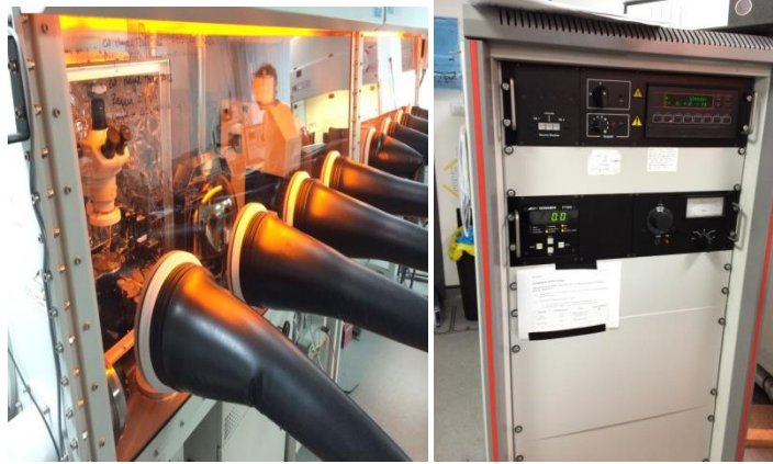
Figure 3.5: Specialized glove box for gold evaporation and deposition of contacts through shadow mask.
