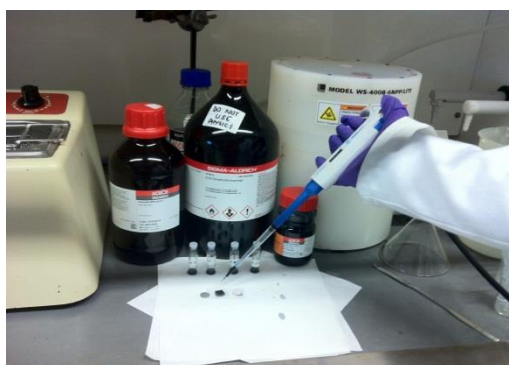
Figure 3.4: Drop casting TIPS-PEN solution with different composition of anisole and decane on Si wafer.
