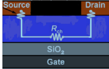
Figure 2.8: Schematic diagram for Top contact bottom gate TFT describing channel and interface resistance (left arrow).
