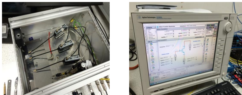
Figure 3.6: Image of microprobe station and semiconductor device analyser (at the School of Chemistry)
