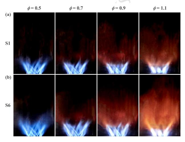
Figure 2: Global flame images of (a) high (S1) and (b) moderate (S6) H<sub>2</sub>-rich syngas at different equivalence ratios.
