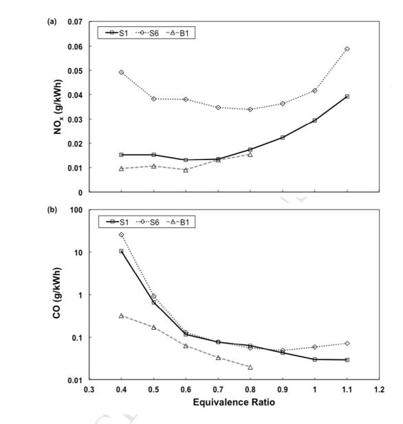
Figure 3: Emissions indices of (a)  $NO_x$  and (b) CO for high  $H_2$ -rich syngas (S1), moderate  $H_2$ -rich syngas (S6) and baseline pure hydrogen syngas (B1) as a function of equivalence ratio.
