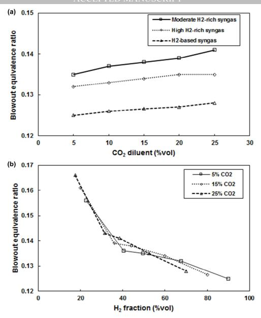
Figure 7: Lean blowout limit (a) for high (S1-S5) and moderate (S6-S10)  $H_2$ -rich syngases compared against baseline (B1-B5)  $H_2$  flames and (b) as a function of percentage of  $H_2$  fraction in syngas at different  $CO_2$  diluent ratios.
