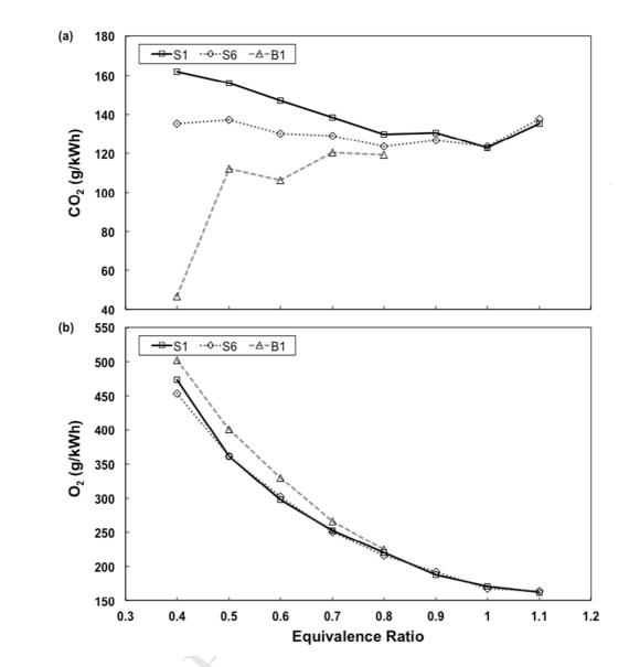
Figure 4: Emission indices of (a)  $CO_2$  and (b)  $O_2$  for syngas S1, S6 and baseline B1 as a function of equivalence ratio.
