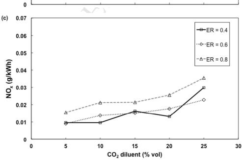
Figure 5: Emission indices of  $NO_x$  for (a) moderate (S6-S10) and (b) high  $H_2$ -rich syngas (S1-S5) and (c) baseline hydrogen (B1-B5) at different  $CO_2$  dilutions and equivalence ratios.
