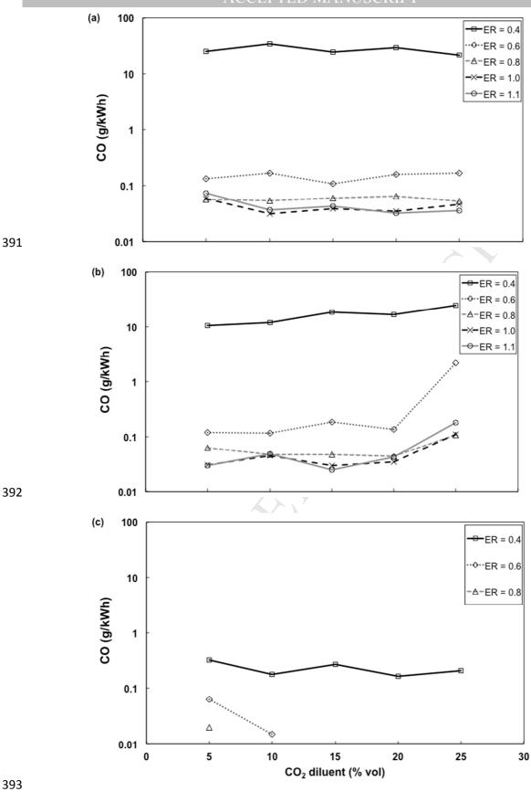
Figure 6: Emission indices of CO for (a) moderate (S6-S10) and (b) high  $H_2$ -rich syngas (S1-S5) and (c) baseline hydrogen (B1-B5) at different  $CO_2$  diluent ratios and equivalence ratios.
