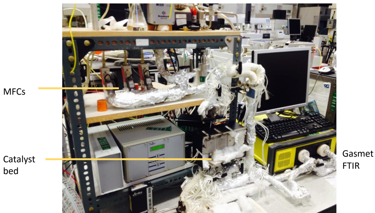
Figure 2.9 Photograph of the water-gas shift reactor
