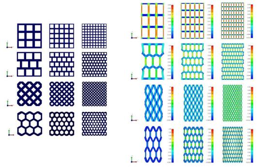
Figure 1. Undeformed model structures with different cell geometries and increasing number of cells while the volume of solid material is fixed (left) and deformed structures subject to 50% stretch in the vertical direction, showing the non-homogeneous Green-Lagrange vertical strains (right). For stacked and diamond cells, the ratio between the thickness and the length of the cell walls also remains unchanged, while for staggered and hexagonal cells, this ratio increases slightly.
