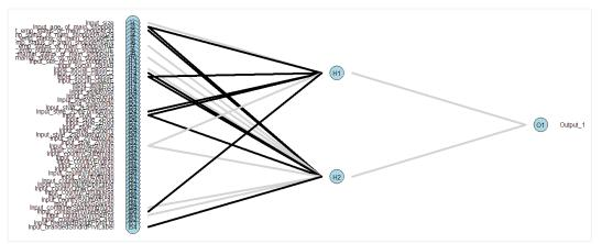
Figure 27. Connectionist network 54-2-1 architecture using consumer data with a single hidden layer and 2 neurons, 1000 iterations, pruning with 100 retrain cycles.
