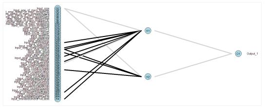
Figure 28. Connectionist network 54-2-1 architecture using consumer data with a single hidden layer and 2 neurons, 10 000 iterations, pruning with 100 retrain cycles.
