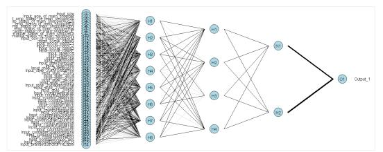
Figure 12. Connectionist network 54-8-4-2-1 architecture using consumer data with 3 hidden layers and 8-4-2 hidden neurons, 1000 iterations, no pruning.
