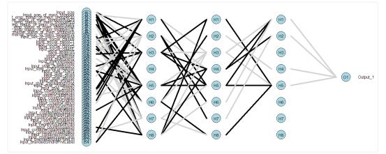
Figure 19. Connectionist network 54-8-8-1 architecture using consumer data with 3 hidden layers and 8 neurons each, 1000 iterations, pruning with 100 retrain cycles.
