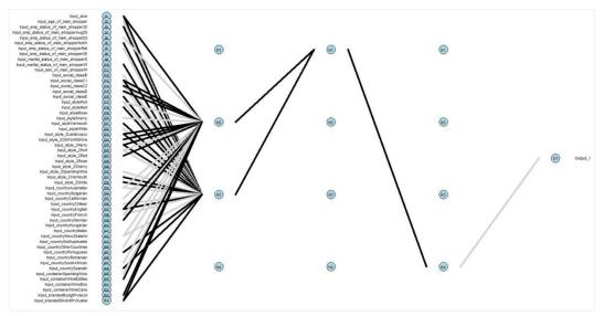
Figure 22. Connectionist network 54-4-4-1 architecture using consumer data with 3 hidden layers and 4 neurons each, 10000 iterations, pruning with 100 retrain cycles.
