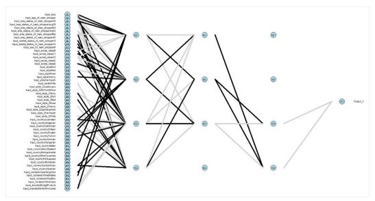
Figure 23. Connectionist network 54-4-4-1 architecture using consumer data with 3 hidden layers and 4 neurons each, 10000 iterations, pruning with 100 retrain cycles.
