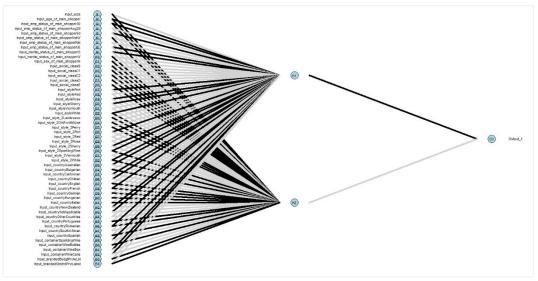
Figure 29. Connectionist network 54-2-1 architecture using consumer data with a single hidden layer and 2 neurons, 10 000 iterations, no pruning.
