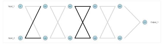
Figure 14. Connectionist model with 2-2-2-2-1 architecture design, no pruning used in model development.
