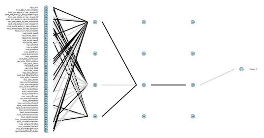
Figure 32. Connectionist network 54-4-4-1 architecture using consumer data with 3 hidden layers and 4 neurons each, 100 000 iterations, pruning with 100 retrain cycles.
