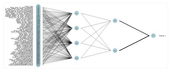
Figure 11. Connectionist network 54-4-2-1 architecture using consumer data with 2 hidden layers and 4-2 hidden neurons, 1000 iterations, no pruning.
