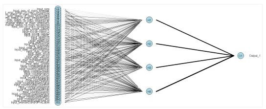
Figure 10. Connectionist network 54-4-1 architecture using consumer data with a single hidden layer and 4 neurons, 1000 iterations, no pruning.
