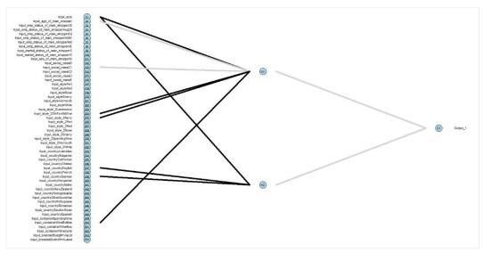
Figure 30. Connectionist network 54-2-1 architecture using consumer data with a single hidden layer and 2 neurons, 10 000 iterations, pruning with 100 retrain cycles.
