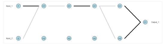
Figure 15. Connectionist model with 2-2-2-2-1 architecture design, pruning used in model development.
