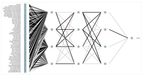
Figure 21. Connectionist network 54-4-4-1 architecture using consumer data with 3 hidden layers and 4 neurons each, 10000 iterations, no pruning.
