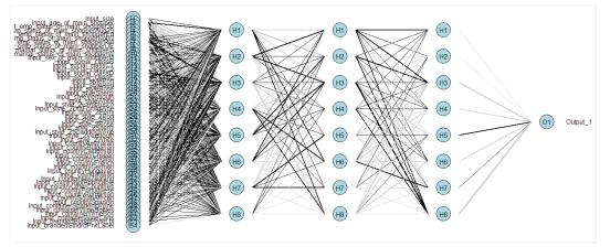
Figure 17. Connectionist network 54-8-8-1 architecture using consumer data with 3 hidden layers and 8 neurons each, 100 000 iterations, no pruning.
