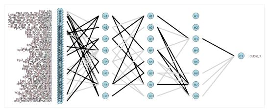
Figure 20. Connectionist network 54-8-8-1 architecture using consumer data with 3 hidden layers and 8 neurons each, 1000 iterations, pruning with 250 retrain cycles.
