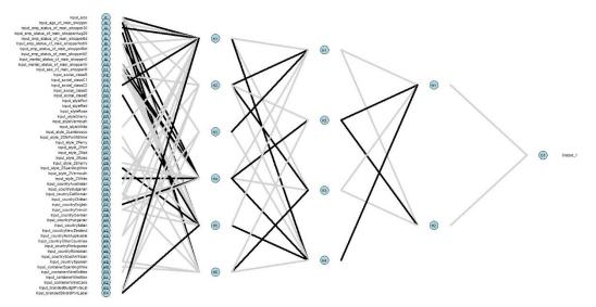
Figure 24. Connectionist network 54-6-4-2-1 architecture using consumer data with 3 hidden layers and 4 neurons each, 10000 iterations, pruning with 100 retrain cycles.
