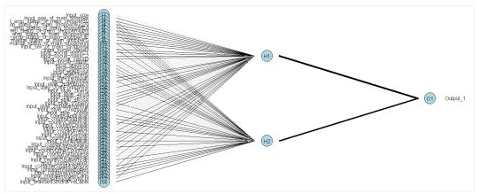
Figure 9. Connectionist network 54-2-1 architecture using consumer data with a single hidden layer and 2 neurons, 1000 iterations, no pruning.
