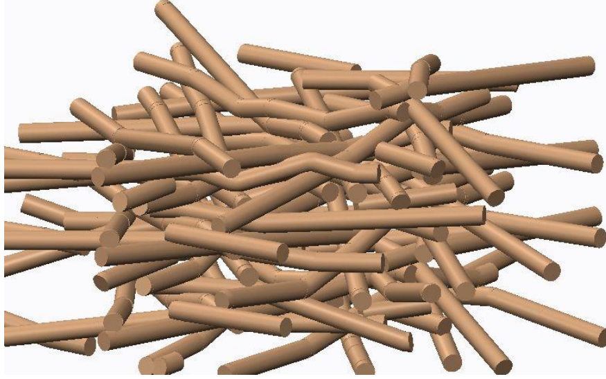
Figure 3.8. The three-dimensional stochastic beam model with polylines developed in this study
