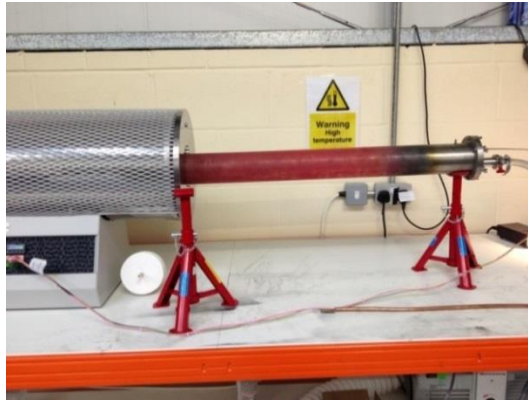
Figure 9. An image showing the vacuum system once a brazing trial has been completed during the cooling phase.
