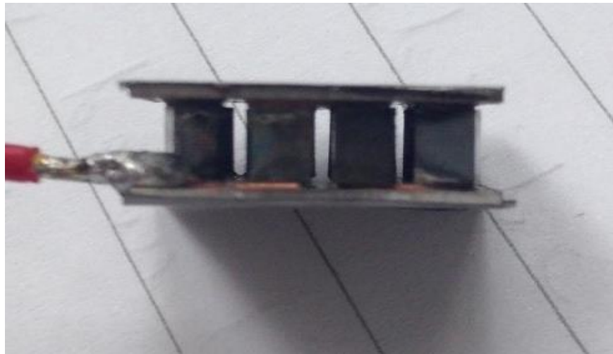
Figure 65. 7-couple silicide module made using Toyota/Yasunaga semiconductor material.
