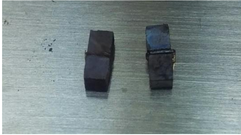
Figure 109. Two Ti/TiN brazed uncouples showing surface degradation after processing.
