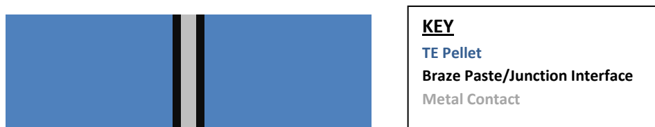
Figure 4. Schematic of the uni-junction design. The key on the right-hand side outlines the specific parts with the colour on the schematic.
