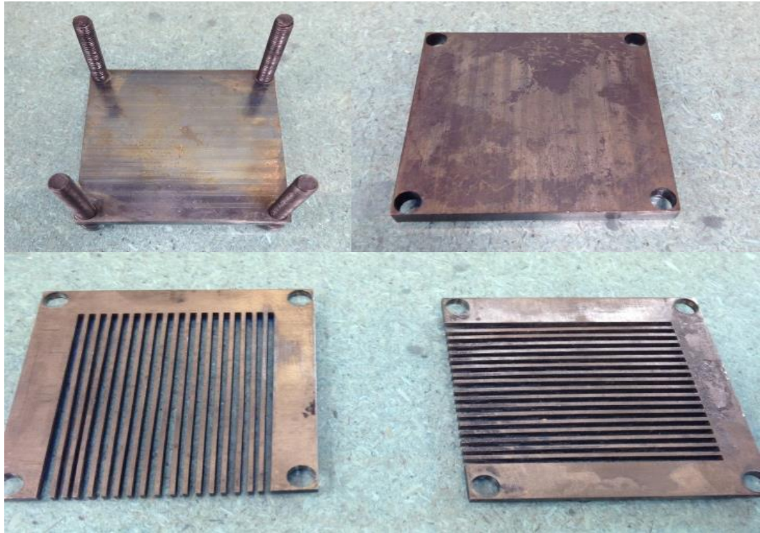
Figure 12. Components of a ‘comb’ style jig. The fingers are positioned at a 90° pitch to provide the ‘checkerboard’ arrangement to position the pellets on the metallised ceramic.
