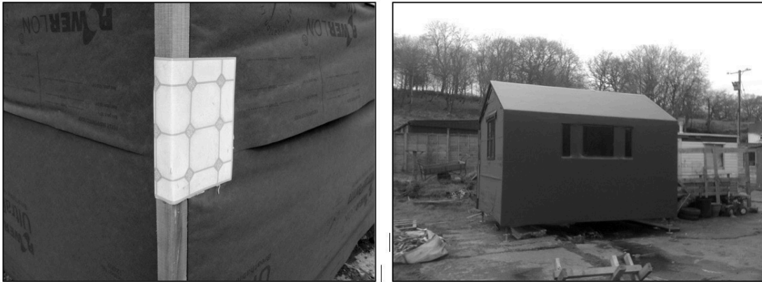
Fig. 6.44 Self-adhesive vinyl floor tile discovered on site used to test idea for cladding (left); and the pod after it had been clad in self-adhesive signage vinyl, but before it began to fail (right)
