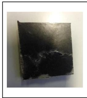
**Figure 16.** Resulting crack on the internal face of the turbine blade.
