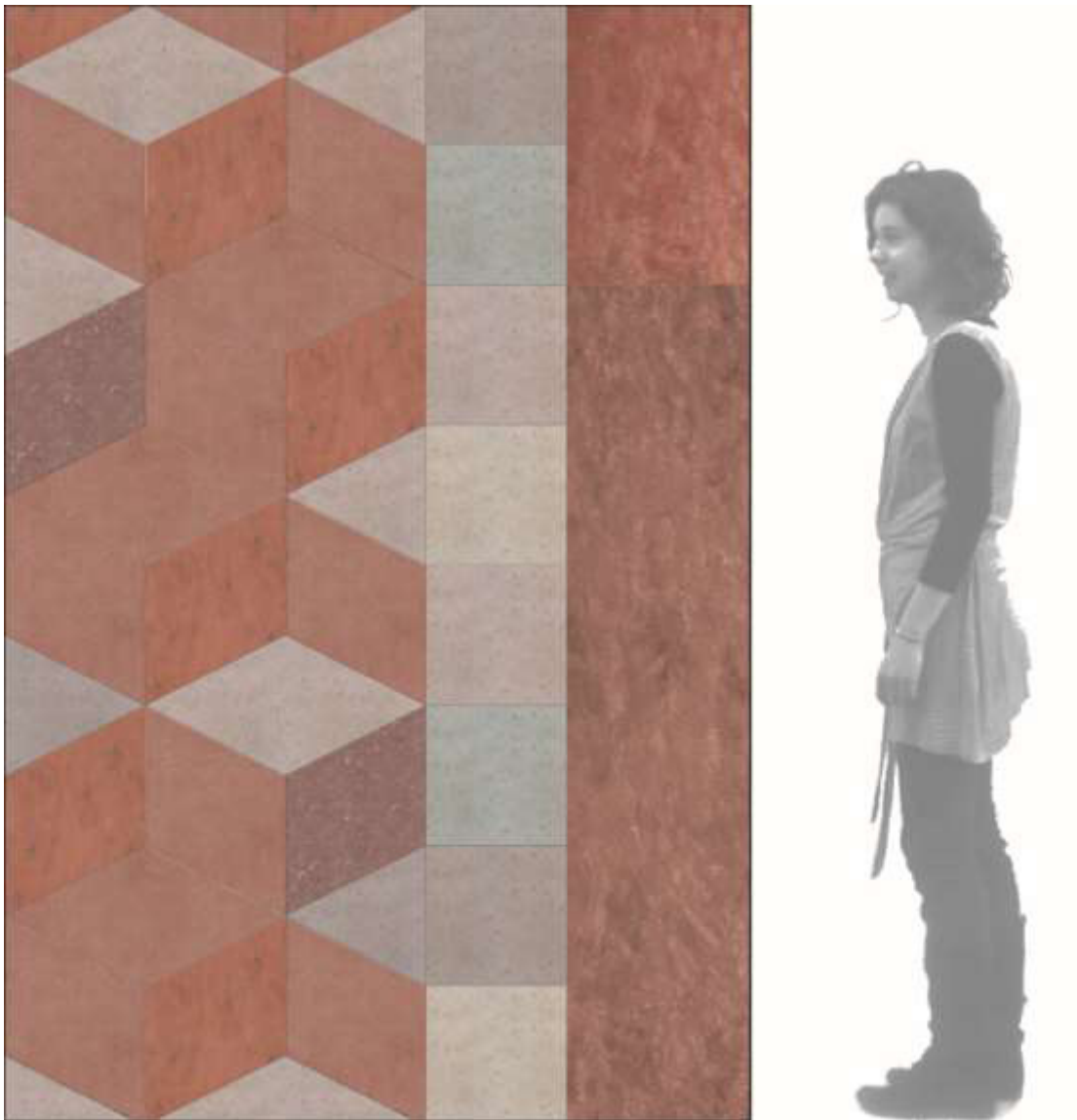
Fig. 8.6 - '176 - Sample Panel'. Design development drawing of the decorative stone cladding façade of the Museum of Childhood, Caruso St John Architects, 2005.
