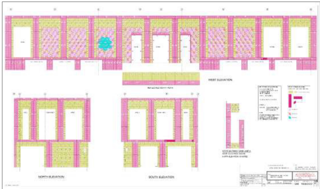
Fig. 8.23 - Shop Drawing of Stonework. Drawing 1909/GA/01 stone key layout to west, north & south elevations. Museum of Childhood. Issued August 2006 / amended 7/9/06; 14/9/06; 1/11/06. Stone Restoration Services.
