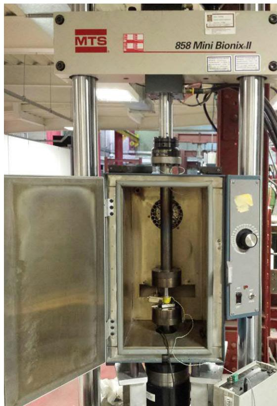
**Figure 5.11 - Test rig with high temperature modifications**
