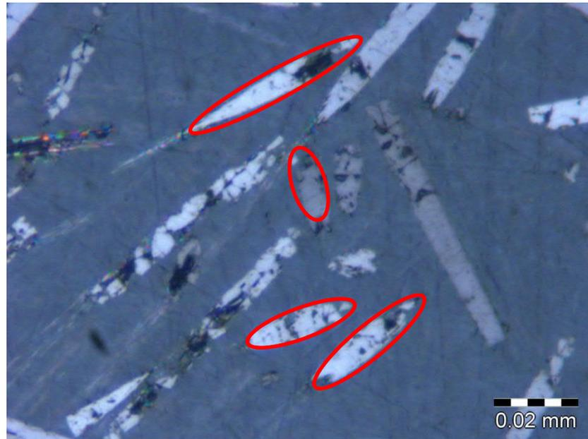
**Figure 6.19 - Optical microscope image of 30%w/w carbon fibre filled PEEK at 320x magnification showing fibre alignment**
