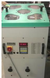
**Figure 4.10 - Arburg Thermolift material dryer**
