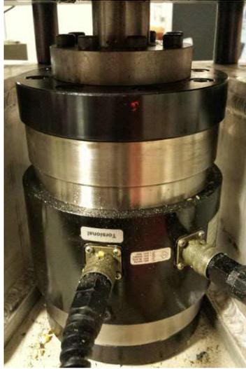
**Figure 5.5 - MTS 858 Mini Bionix II Fixed Half & Load Cell**
