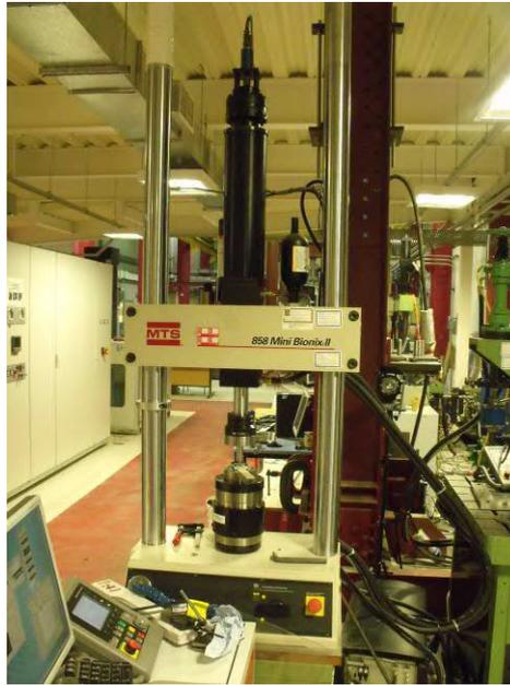
**Figure 5.4 - MTS 858 Mini Bionix II Test Apparatus**
