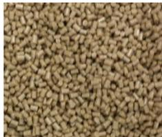
Figure 4.2 - PEEK pellets for injection moulding
