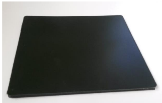
Figure 2.13: An example of 1 mm microvaristor compound based silicone rubber [11].
