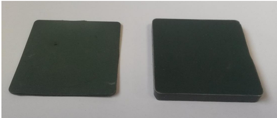
Figure 4.9: The non-linear microvaristor A composite samples that were obtained at different microvaristor concentrations and thicknesses. The sample of 1 mm with 60 wt. % (left) and of 5 mm with 70 wt. % (right).
