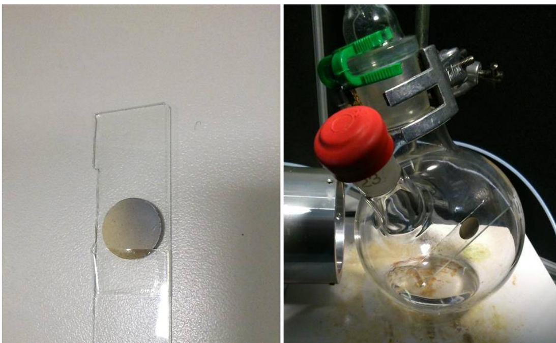
Figure 10. Left, image of an 8 mm diameter 3wt% Pd-C<sub>3</sub>N<sub>4</sub> pellet (100 mg made by incipient wetness) attached to a glass slide. Right, image of the glass slide with pellet attached inside the photo reactor with the pellet held above the liquid at the bottom.
