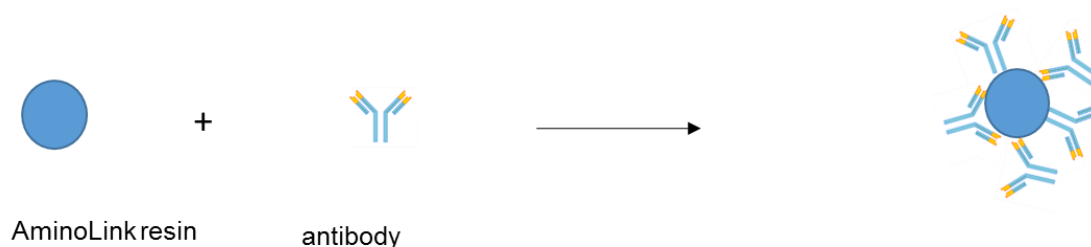
Figure 91. Direct antibody immobilisation IP, without cross-linker. The epitope of the antibody may be masked due to their untidy orientation.
