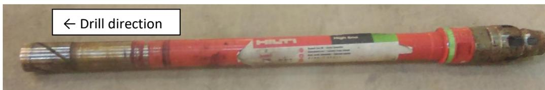
Figure 4.2: Image of the diamond core drill
