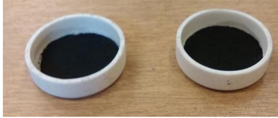
Figure 4.5: Crucibles for determining the moisture and ash content
