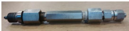
Figure 3.13: Equipment which was used to connect the right screw cap end of the reactor with the gas line
