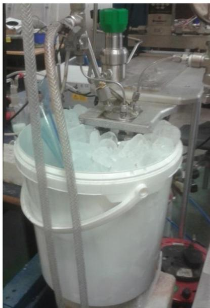
Figure 4.8: The tar trap put into a bucket with ice cubes to drop its temperature
