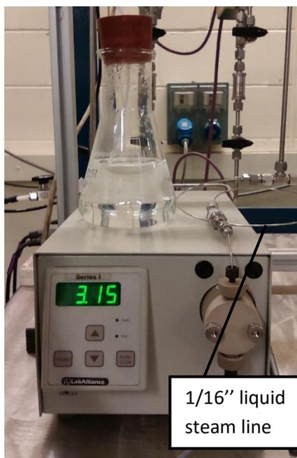
Figure 3.5: The HPLC pump with a glass bottle filled with deionised water
