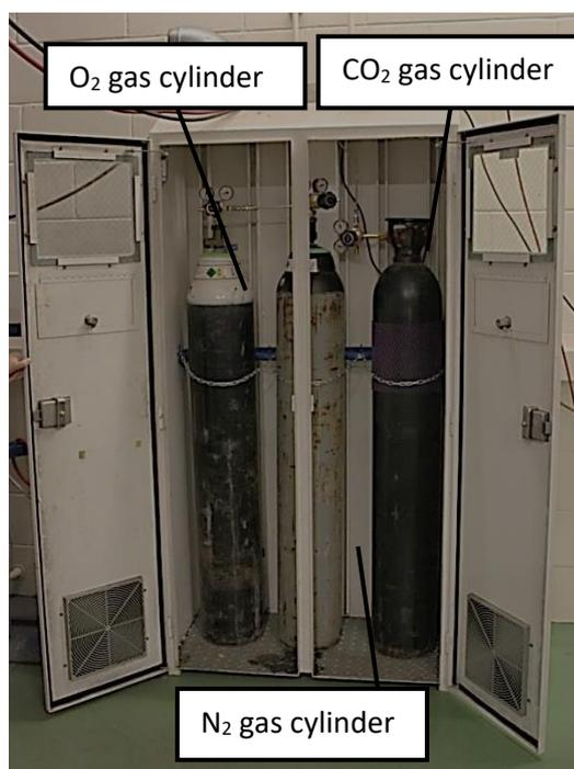
Figure 3.3: The cylinder cupboard with the O<sub>2</sub>, CO<sub>2</sub> and CO gas cylinders
