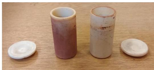
Figure 4.6: Crucibles for determining the volatile matter
