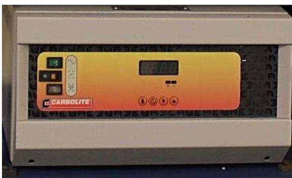
Figure 3.16: Temperature controller of the Horizontal Split Tube (HST) furnace.
