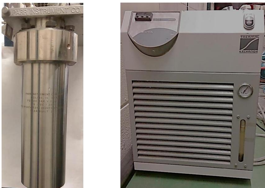
Figure 3.18: The gas liquid separator (tar trap) (on the left) and the cooler (on the right)
