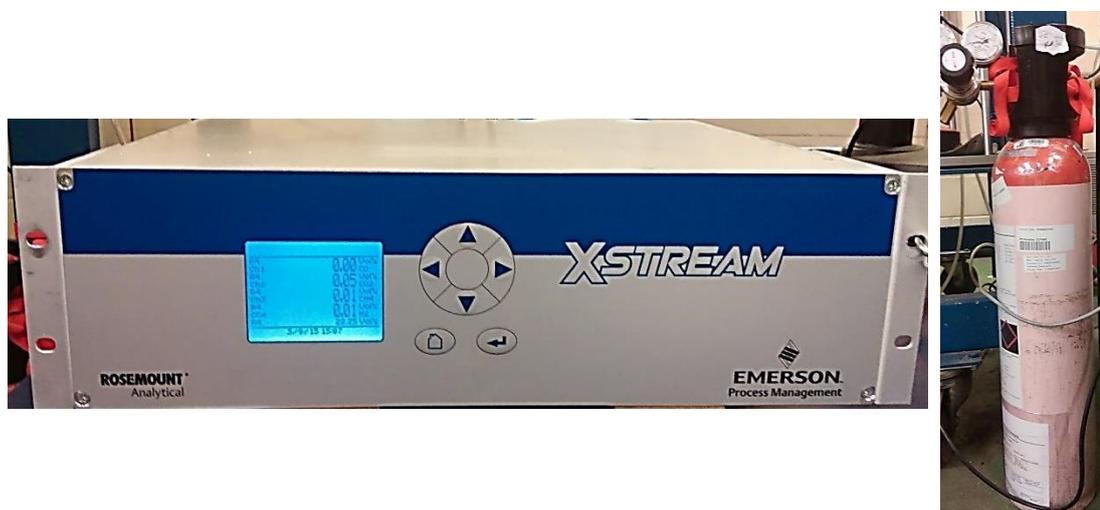
Figure 3.21: The X-Stream Enhanced XEGP-General Purpose Gas Analyser (left) and its calibration gas (right)
