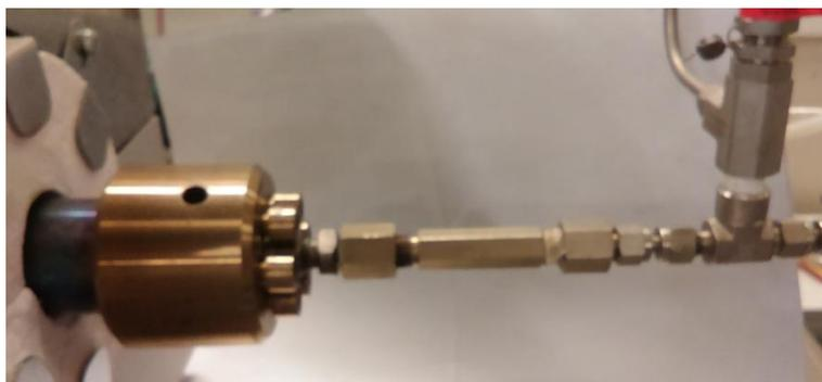
Figure 3.14: The right screw cap ending of the reactor connected to the gas line
