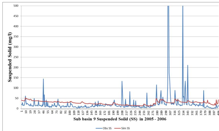
**Figure 5-4 Sediment Calibration Hydrograph at River Piddle (2005-2006)**
