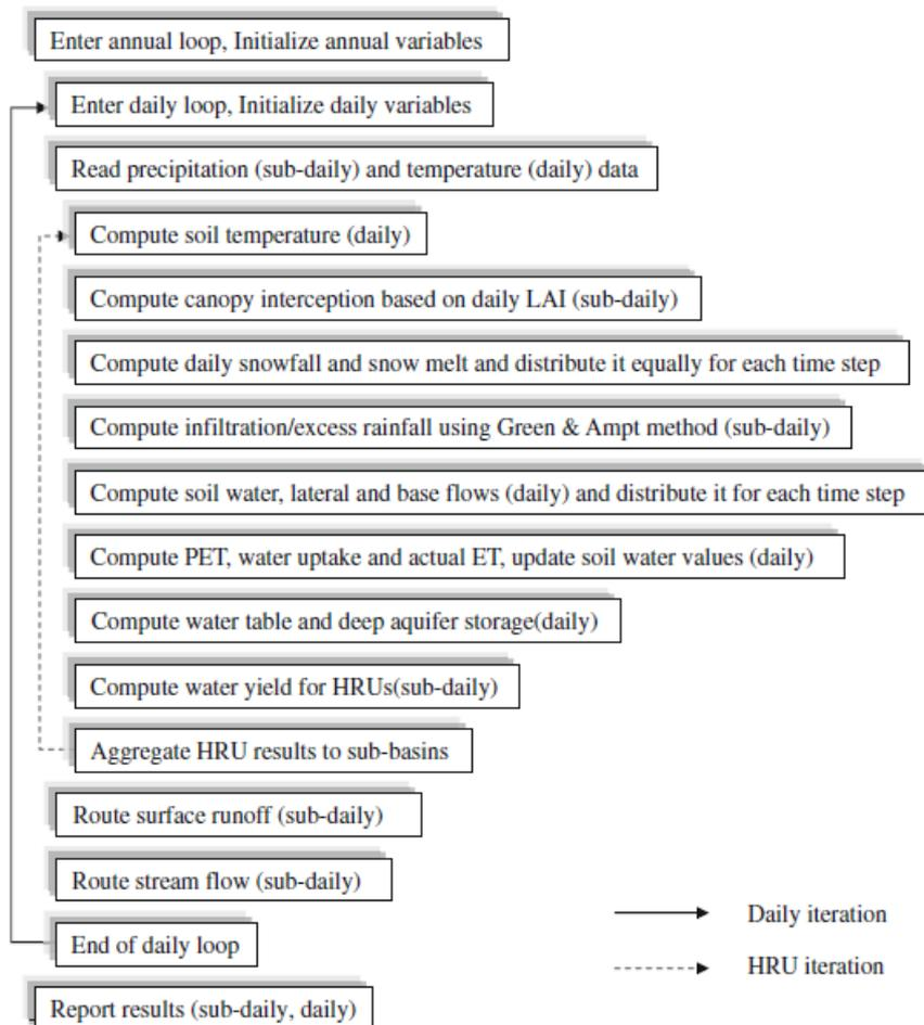
**Figure 4-7 Flow Chart of Daily and Sub-daily Flow Routing in SWAT (Neitsch, Arnold et al. 2005)**
