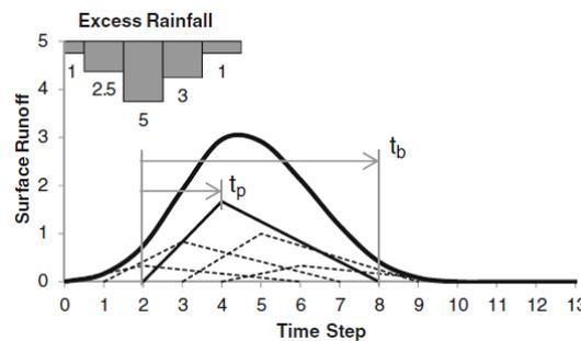
**Figure 4-9 Triangular Unit Hydrograph (Neitsch, Arnold et al. 2005)**
