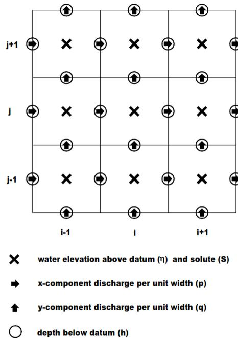
Figure 7-2 Illustration of Space Staggered Grid System (Falconer 2001)
