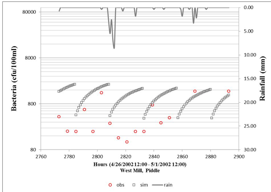
**Figure 5-14 (a) Storm Event Validation with Solar Radiation Inactive, Piddle (2002)**
