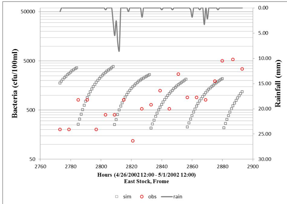
**Figure 5-15 (a) Storm Event Validation with Solar Radiation Inactive, River Frome**
