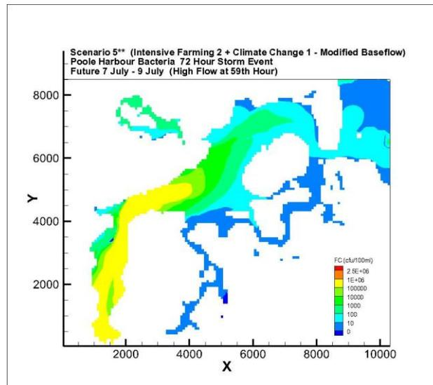
**Figure 7-7 (a) Scenario 5 Bacteria with Modified Base Flow at Low Tide**
