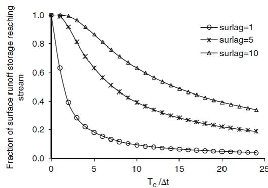
**Figure 4-8 Surface Lag Impact to Main Channel (Neitsch, Arnold et al. 2005)**
