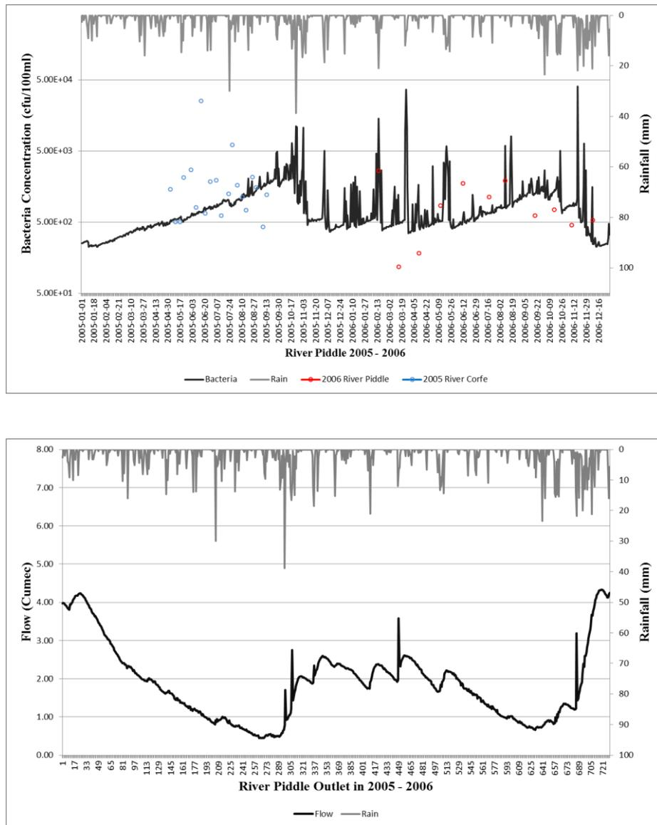
**Figure 5-5 (a) Bacteria calibration at Piddle outlet (daily) (b) Flow at Piddle outlet**
