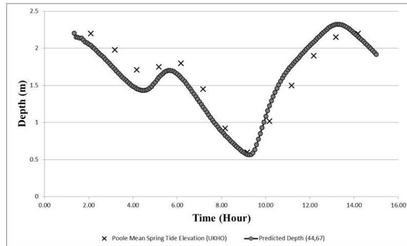
**Figure 7-3 Validation of Water Elevation during Spring Tide**
