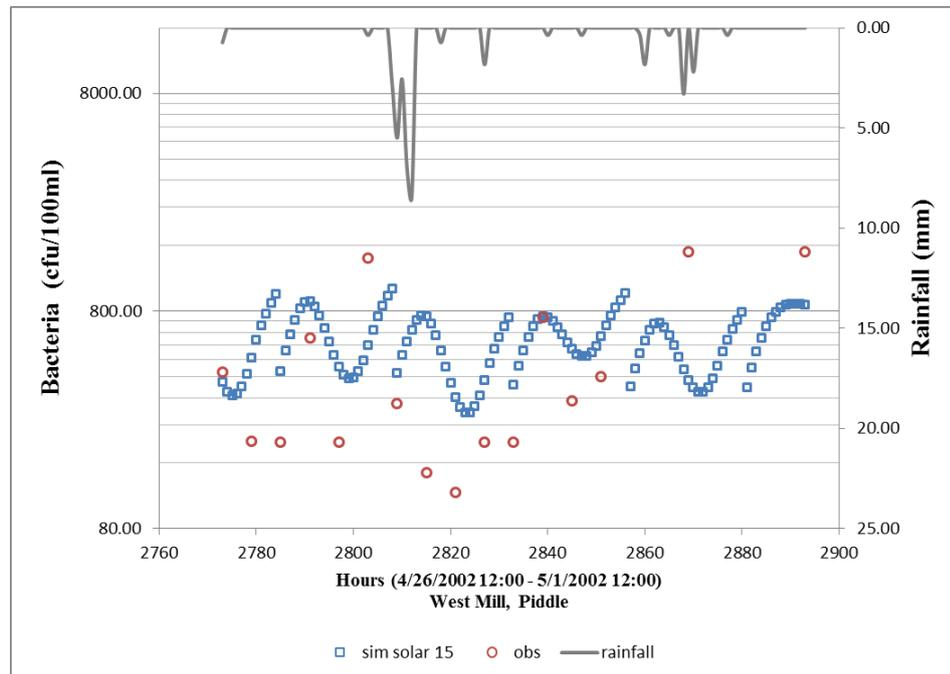
**Figure 5-14 (c) Storm Event Validation with Solar Radiation Activate, Piddle (LDLPRCH = 15)**
