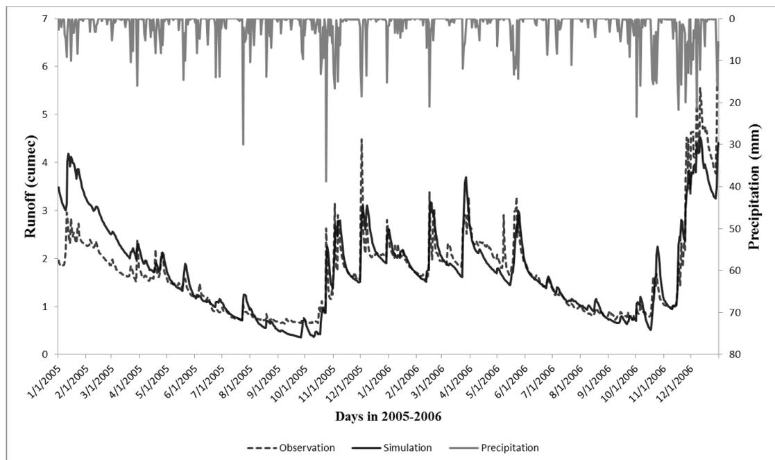
Figure 4-10 (b) Flow Calibration Sub - basin 8 (2005-2006)
