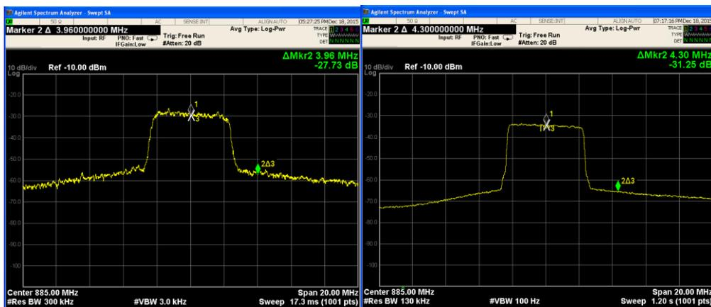
Figure 5.8 - Spectral display of the output signal before (left) and after (right) applying DPD.
