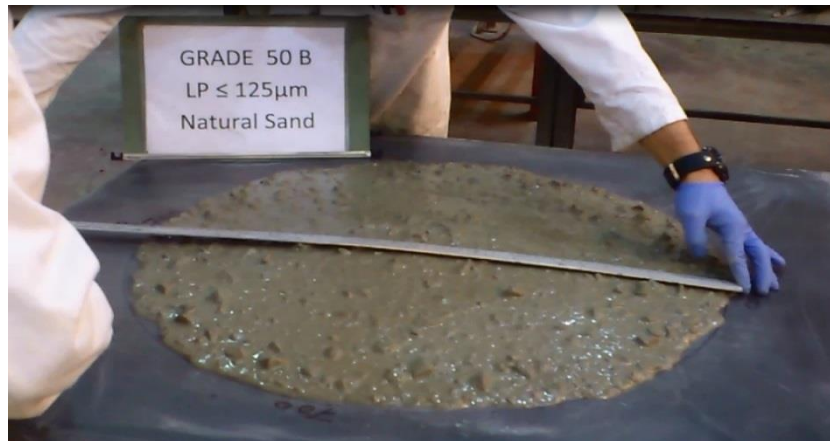
Figure 5. 6 Horizontal spread of SCC mix (Natural fine aggregate replacements by coarser limestone filler)
