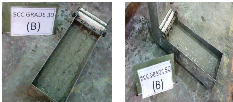
Figure 5. 16 Passing and filling of SCC Mix 30MPa (left) and 50MPa (right)
