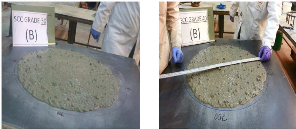
Figure 5. 3 Horizontal spread of SCC Mix 30MPa
