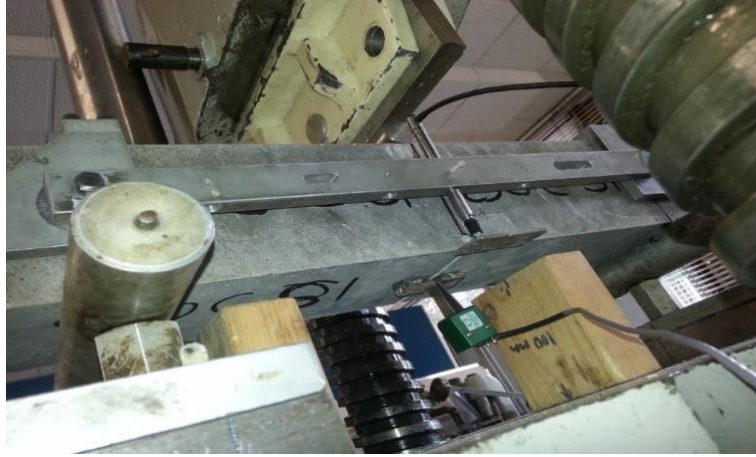
Figure 6. 4 Beam specimen used for TPB test
