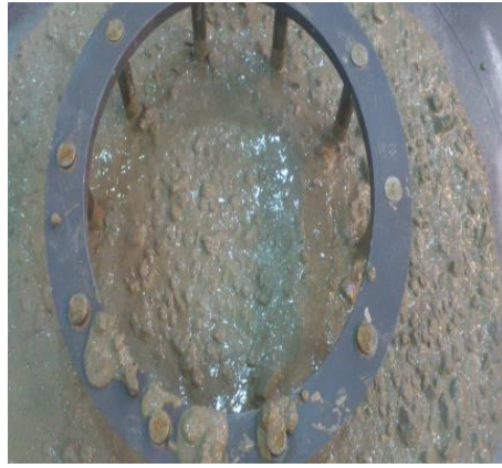
Figure 5. 13 Top-view of the passing ability (J-ring test)
