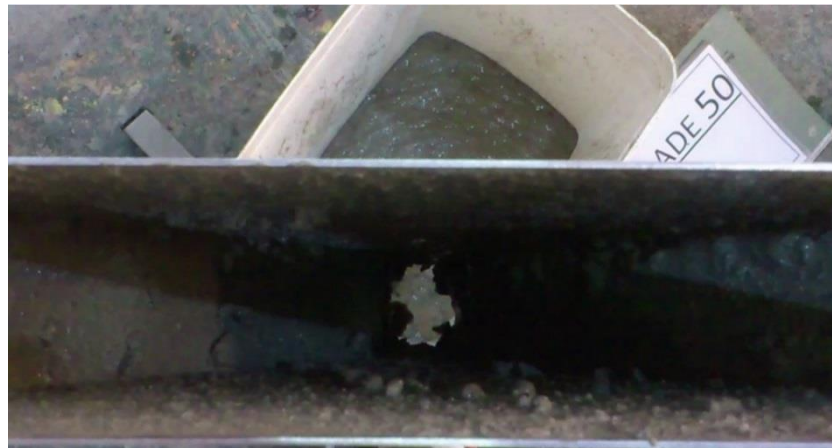
Figure 5. 2 Recording V-funnel time (daylight appearing when viewed from above)
