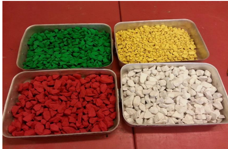
Figure 7. 2 Colour coded coarse aggregates; g \geq 20 mm (white, bottom right), 16 \leq g < 20 mm (red, bottom left), 12 \leq g < 16 mm (green, top left), and 8 \leq g < 12 mm (yellow, top right)
