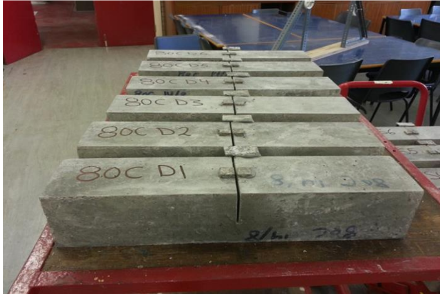
Figure 6. 7 The hardened SCC deep-notched beams
