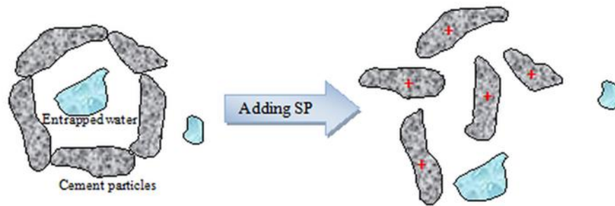
Figure 2. 3 Method of deflocculation and water liberation with use of Super-plasticiser, (After: Deeb, 2013)
