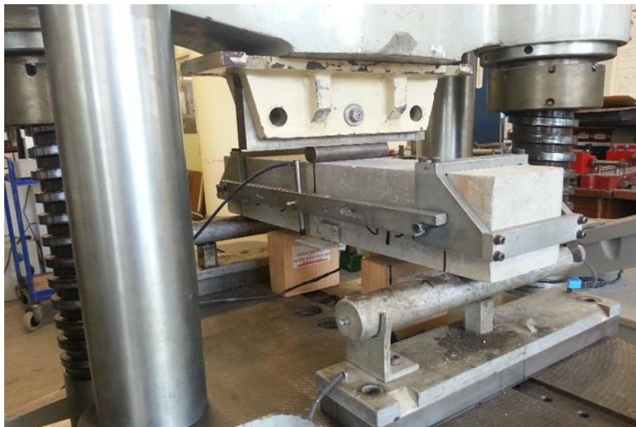
Figure 6. 8 The TPB ready for testing
