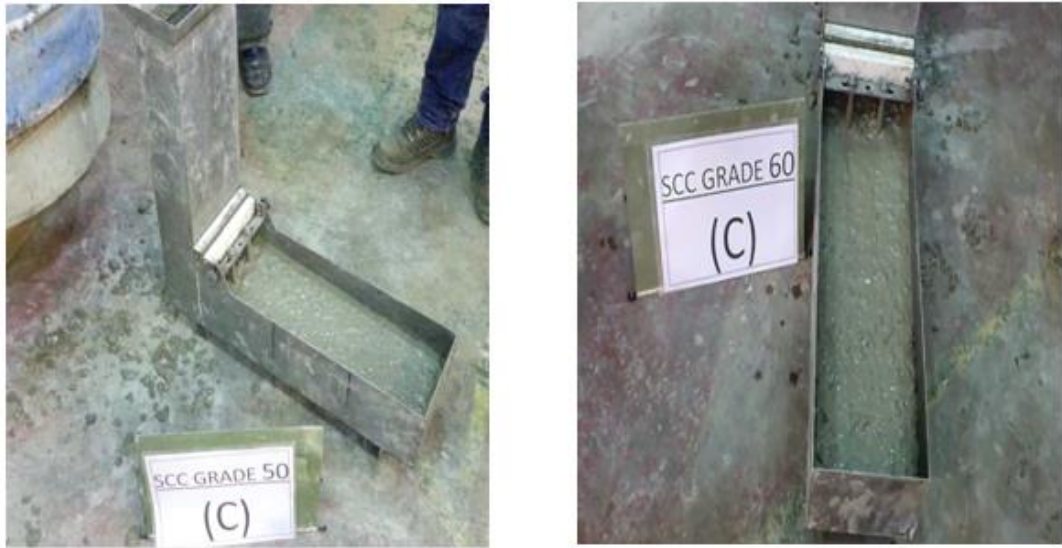
Figure 5. 17 Passing and filling of SCC mix: 50C (Left), 60C (Right)
