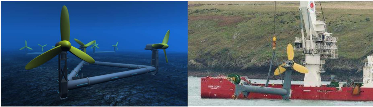
Figure 1.12 Tidal Energy Limited a) DeltaStream concept b) Full-scale turbine demonstration (Tidal Energy Ltd, 2016)
