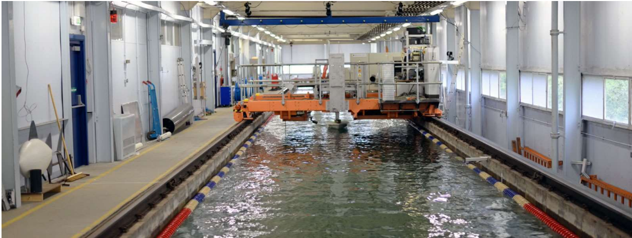
Figure 2.5 Kelvin Hydrodynamics Laboratory Towing Tank (Univeristy of Strathclyde, 2012)
