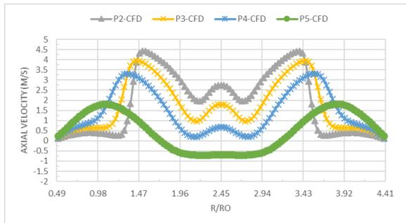
**Figure 5.** Axial velocity at different planes from burner mouth, 600 LPM tangential inlet, X=150 mm with air injection effect
