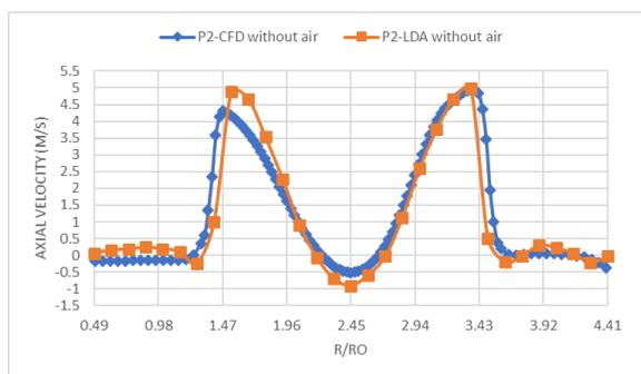
**Figure 2:** Comparison of axial velocity measured by LDA with CFD result at P2, 600 LPM tangential inlet, X=150 mm and no air injection
