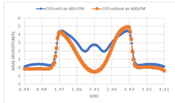
**Figure 3.** Effect of axial air injection on the defect of axial velocity at P2 with X = 150 mm, 600 LPM tangential inlet
