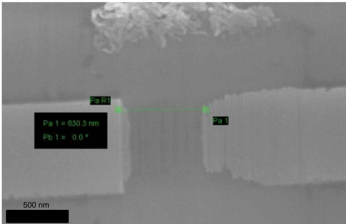
**Figure 5-12 Showing an SEM image of nanowire 1 (10nm thick), after the final machining attempt which destroyed the wire.**
