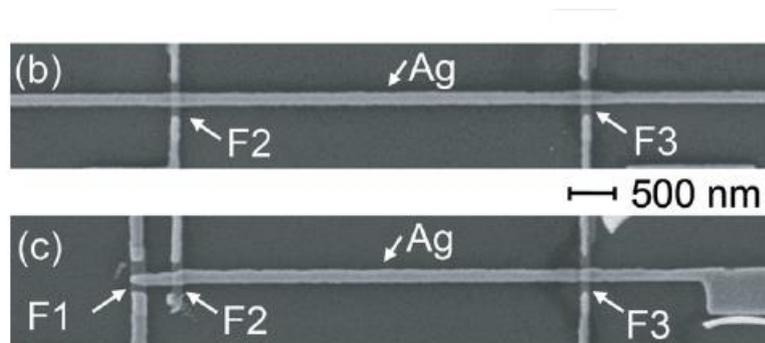
**Figure 2-13** showing a standard lateral spin valve with only one injecting electrode (top image) and a dual lateral spin valve with two electrodes for injecting the spin current and a reduced volume for spin relaxation. Image adapted from reference [33]
